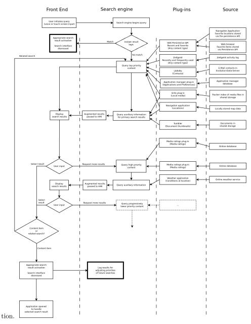
If this logic completes the search, the appropriate action is taken and the interface is dismissed. If there is no user selection within a configurable time, the search engine begins performing queries of the back end plug-ins, starting with the highest priority information categories (static data content), including auxiliary information.
