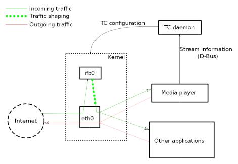
To demonstrate the functionality as describe above a simple demonstration media application using Gstreamer will be written that communicates with the Traffic control daemon in the manner described. Furthermore some a testcase will be provided to emulate changing network conditions.
