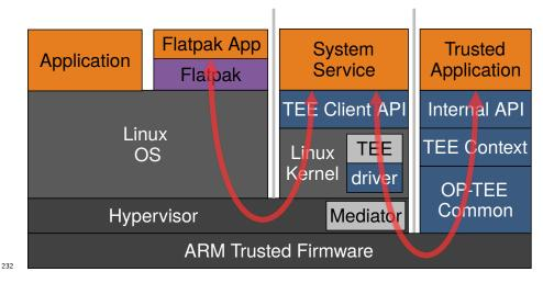
For example, rather than each Flatpak downloading encrypted downloads and passing the content of these to a TA to decrypt via a TEE proxy, a system service could be provided to download, validate and decrypt files for the Flatpak apps. This would be advantageous as it would reduce the number of hops that data would need to take from being downloaded to being available in the container decrypted, improving device efficiency.
