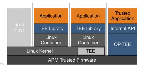
We expect that calls between the containers and TEE would work, however unlike when virtualization is utilized, the TEE will not provide a separate context for each of the REEs and as such it is likely that, depending on the trusted applications installed, it might be possible for some data to leak between the containers via the TEE.
